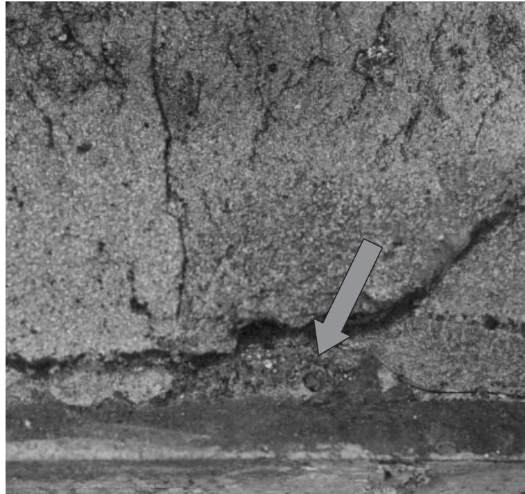
Fig. 4. Ductile tearing at root of predominantly cleavage fracture.
